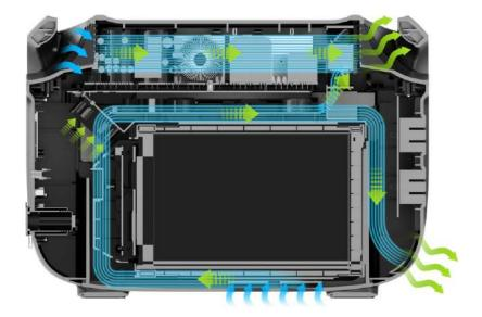
The product is a portable energy storage power supple with a built-in-high-efficiency power lithium-ion battery, a safe lithium battery management system (BMS), efficient thermal energy enmanagement system (TMS)
